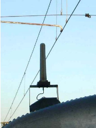
Figure 4: Challenging, but inadequate installation of a train antenna
